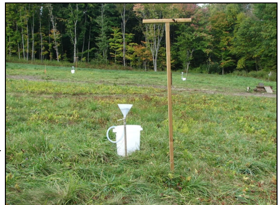
Figure 2. Bulk precipitation collector. The two-liter storage bottle is in the plastic bucket and not visible.
